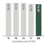
turn in late 2021. Slimes levels in the process increased to levels that interrupted our mine plan, impacting head feed grades and utilisations. The high slimes also reduced process recoveries, overall reducing HMC production.
