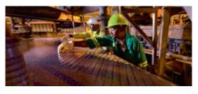
The MSP uses a series of magnetic, gravity and electrostatic separation circuits to separate valuable minerals and to produce various ilmenite, rutile and zircon product grades to meet specific customer requirements.
